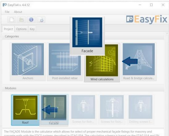
The FAÇADE Module is the calculator which allows for select of proper mechanical façade fixings for masonry and concrete walls with the ETICS systems described in ETAG 004. The calculation schema is based on the ETAG 014 and EN 1991-1-4 Standard.
